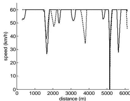
Figure 4. Example of vehicle speed during the test. Solid line: Mobile model, Dashed line: Sphere model.
