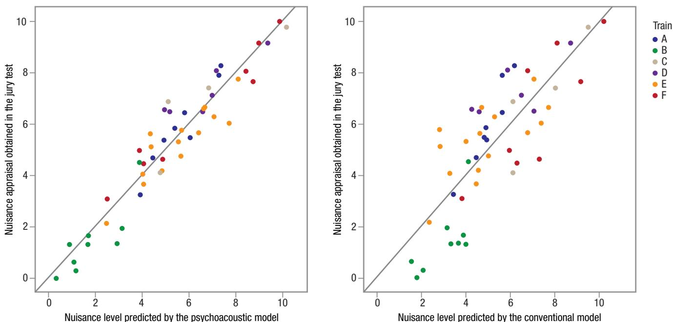
Figure 6. Comparison of the model with psychoacoustic parameters (left) and conventional acoustic parameters (right).
