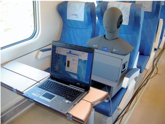
Figure 2. Artificial head placed in the passenger car.
