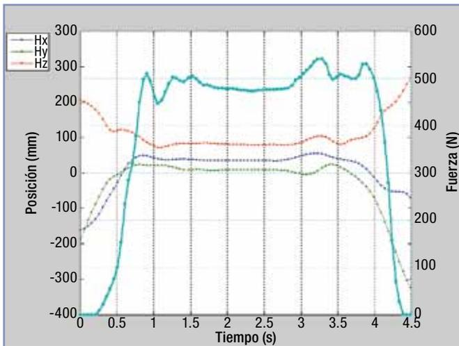
Figure 4. Pattern of force and movement of the H-point.
