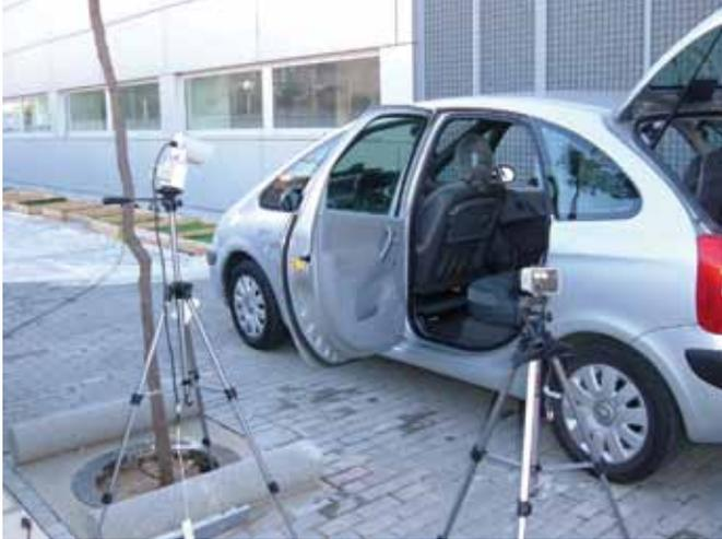
Figure 1. Testing stage and photogrammetry system.
