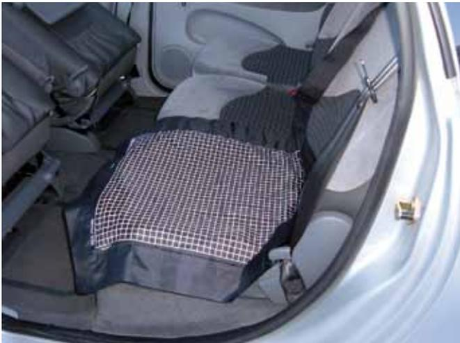
Figure 2. Pressure blanket on seat.
