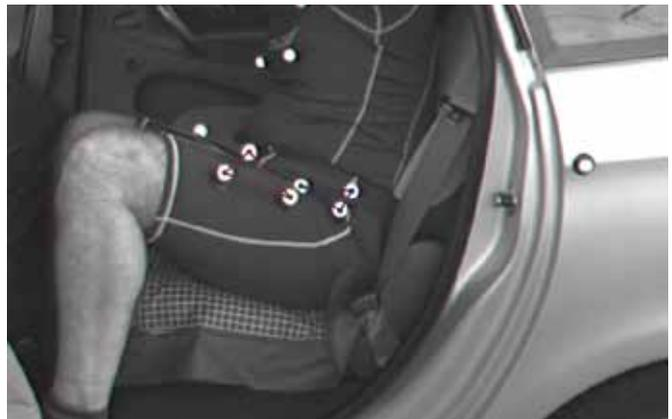
Figure 3. Measurement of the ingress/egress movement.
