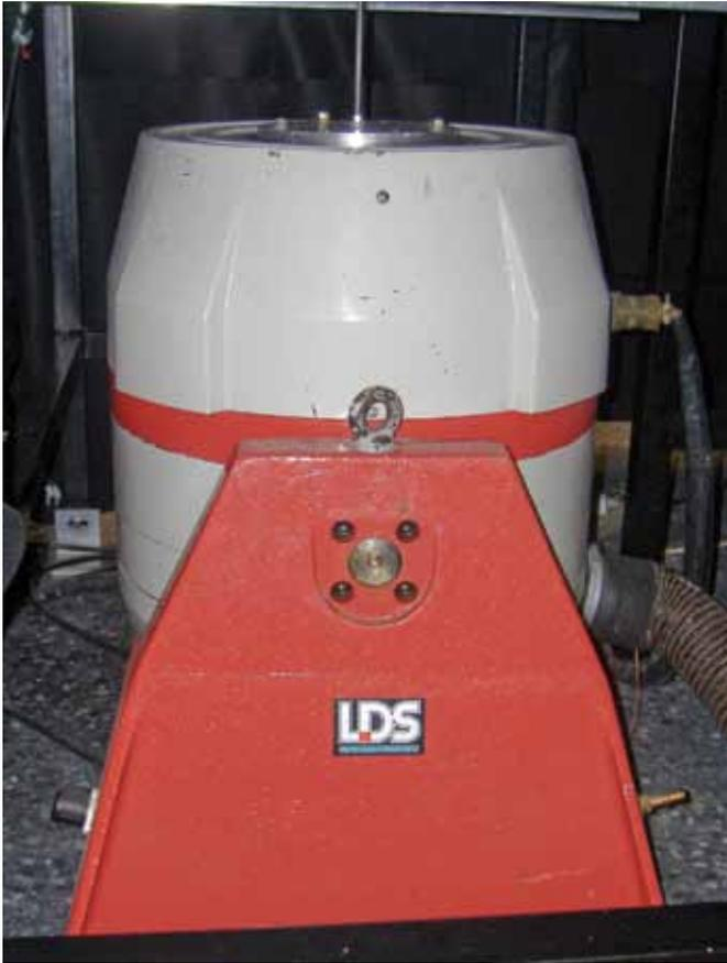
Figure 2. Electrodynamic driver used in the platform.
