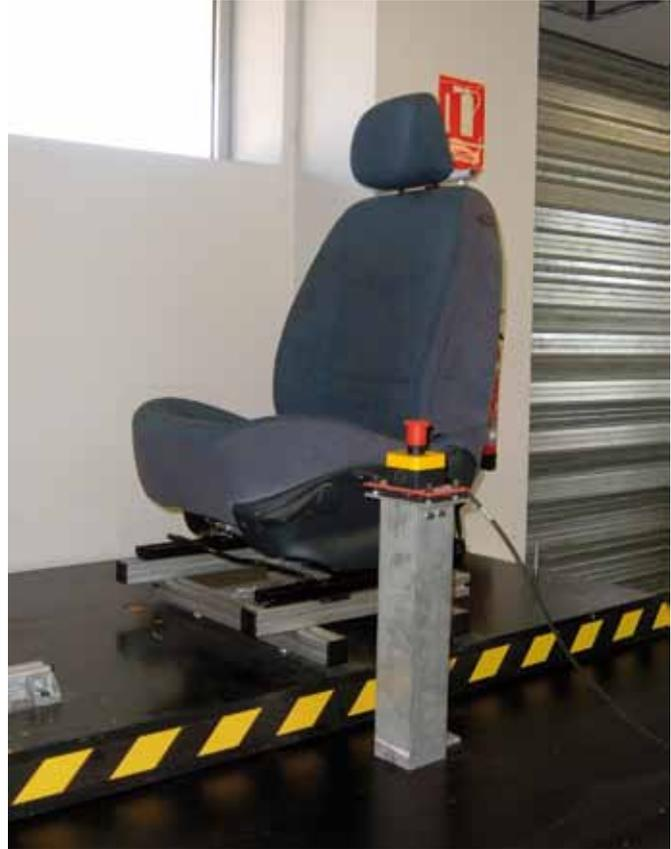
Figure 3. Emergency stop mushroom button within the reach of the test subject.
