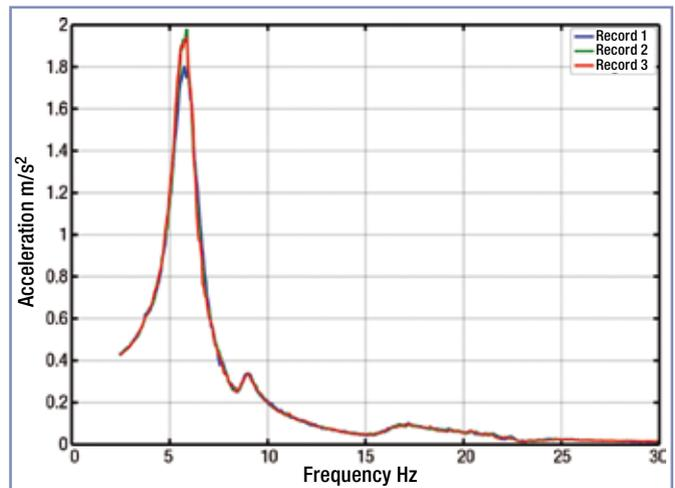
Figure 4. Frequency response function of an automobile seat.
