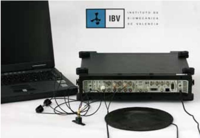
Figure 6. Vibration acquisition device for measuring vibrations in passengers.
