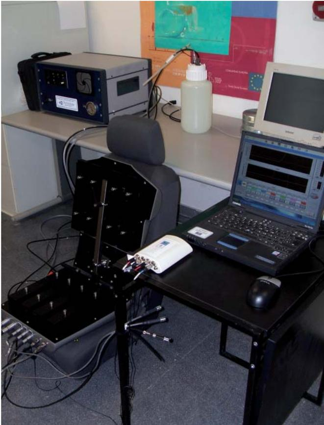
Figure 1. Test with seats in the laboratory using the STAN thermal comfort dummy.
